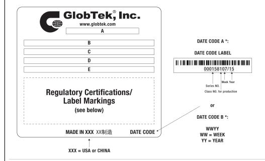
A=ICT / ITE / Medical Power Supply/Class 2/Household Power Supply B=P/N: (料号) TR9KS1111T00CIMR6B C=Model (型号) GTM96600-6054-T2 D=Input (输入)100-240V~, 50-60Hz, 1.5A E=Output (输出)54.0 V == 1.11 A, 60.00W
