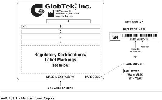
A=ICT / ITE / Medical Power Supply B=P/N: (料号) TR9KR4000T00-IM(R6B) C=Model (型号) GTM961200P12030-T2 D=Input (输入)100-240V~, 50-60 Hz, 1.5 A E=Output (输出)30.0 V === 4.0 A, 120.00W
