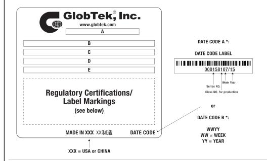
A=ICT / ITE / Medical Power Supply/Class 2/Household Power Supply B=P/N: (料号) TR9KI750LCP-IMR6B C=Model (型号) GTM96180-1830-6.0-T2 D=Input (输入)100-240V~, 50-60 Hz, 0.6 A E=Output (输出)24.0 V == 0.75 A, 18.00W
