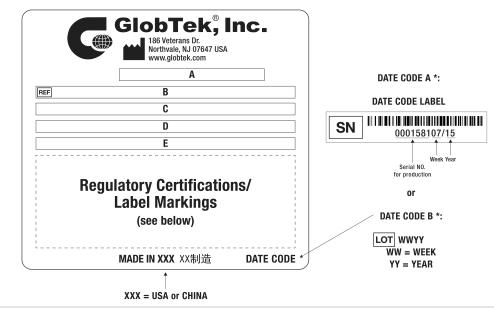
A=Medical/ICT/ITE/Household use Power Supply B=P/N: (料号) TR9KI7500LCPIMR6B C=Model (型号) GTM961800P18024-T2 D=Input (输入)100-240V~, 50-60 Hz, 2.2A E=Output (输出)24.0 V === 7.5 A, 180.00W
