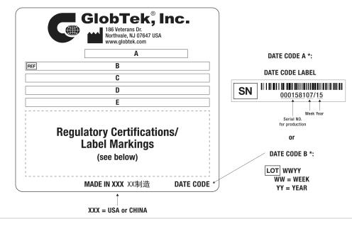
A=Medical/ICT/ITE/Household use Power Supply B=P/N: (料号) TR9KI6666LCPIMR6B C=Model (型号) GTM961600P16024-T2 D=Input (输入)100-240V~, 50-60 Hz, 2.2A E=Output (输出)24.0 V === 6.66 A, 160.00W
