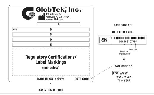
A=Medical/ICT/ITE/Household use Power Supply B=P/N: (料号) TR9KI6666CCPIMR6B C=Model (型号) GTM961600P16024-T2 D=Input (输入)100-240V~, 50-60 Hz, 2.2A E=Output (输出)24.0 V == 6.66 A, 160.00W
