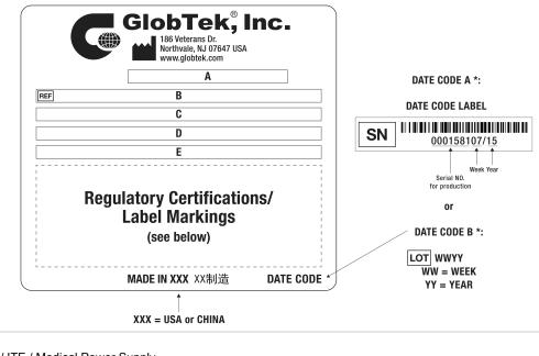
A=ICT / ITE / Medical Power Supply B=P/N: (料号) TR9KI5000LCP-IM(R6B) C=Model (型号) GTM961200P12024-T2 D=Input (输入)100-240V~, 50-60 Hz, 1.5 A E=Output (输出)24.0 V === 5.0 A, 120.00W
