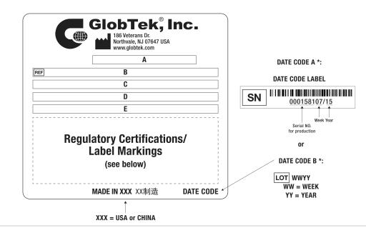
A=ICT / ITE / Medical Power Supply/Class 2/Household Power Supply B=P/N: (料号) TR9KI3750CCP-IM(R6B) C=Model (型号) GTM96900P9024-T2 D=Input (输入)100-240V~, 50-60 Hz, 1.5A E=Output (输出)24.0 V == 3.75 A, 90.00W
