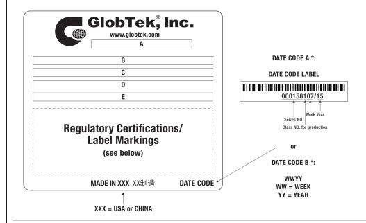
A=ICT / ITE / Medical Power Supply/Class 2/Household Power Supply B=P/N: (料号) TR9KI2700LCPCIMR6B C=Model (型号) GTM96600-6524-T2 D=Input (输入)100-240V~, 50-60Hz, 1.5A E=Output (输出)24.0 V == 2.7 A, 65.00W
