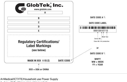
A=Medica//C1/12/Addsenoid use Power Supp B=P/N: (料号) TR9KI1500LCPIMNAR6B C=Model (型号) GTM96300-3624-T2 D=Input (输入)100-240V~, 50-60 Hz, 1A E=Output (输出)24.0 V === 1.5 A, 36.00W
