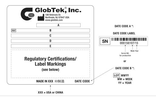
A=Medical/ICT/ITE/Household use Power Supply B=P/N: (料号) TR9KI1500CCPIMNAR6B C=Model (型号) GTM96300-3624-T2 D=Input (输入)100-240V~, 50-60 Hz, 1A E=Output (输出)24.0 V == 1.5 A, 36.00W
