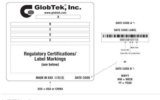
A=ICT/ITE Power Supply B=P/N: (料号) TR9KI1000LCP-N(R6B) C=Model (型号) GT-46240-2424-T2 D=Input (输入)100-240V~, 50-60 Hz, 0.6 A E=Output (输出)24.0 V === 1.0 A, 24.00W
