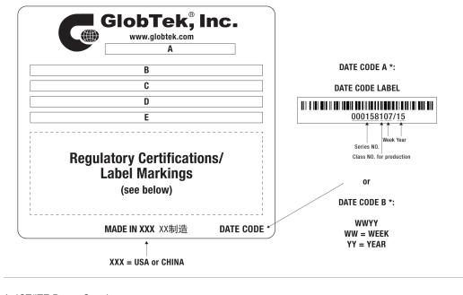
A=ICT/ITE Power Supply B=P/N: (料号) TR9KI1000CCP-N(R6B) C=Model (型号) GT-46240-2424-T2 D=Input (输入)100-240V~, 50-60 Hz, 0.6 A E=Output (输出)24.0 V === 1.0 A, 24.00W
