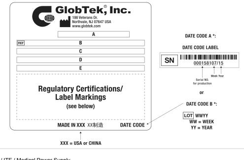
A=ICT / ITE / Medical Power Supply B=P/N: (料号) TR9KH6666LCP-IM(R6B) C=Model (型号) GTM961200P12018-T2 D=Input (输入)100-240V~, 50-60 Hz, 1.5 A E=Output (输出)18.0 V == 6.66 A, 120.00W
