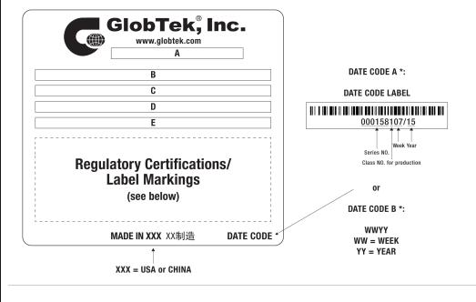
A=ICT/ITE Power Supply B=P/N: (料号) TR9KH2220A00-N(R6B) C=Model (型号) GT-46400-4019-1.0-T2 D=Input (输入)100-240V~, 50-60 Hz, 1.0A E=Output (输出)18.0 V == 2.22 A, 40.00W
