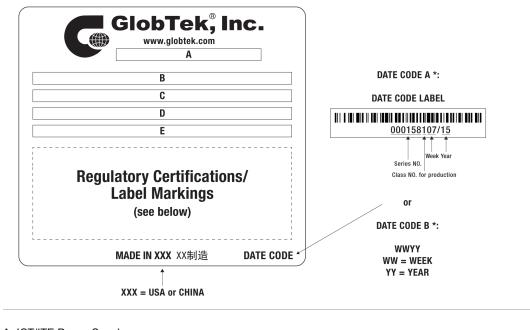
A=ICT/ITE Power Supply B=P/N: (料号) TR9KH1333CCP-N(R6B) C=Model (型号) GT-46240-2424-6.0-T2 D=Input (输入)100-240V~, 50-60 Hz, 0.6 A E=Output (输出)18.0 V === 1.33 A, 24.00W
