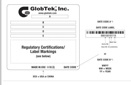
A=ICT/ITE Power Supply B=P/N: (料号) TR9KG2660CCP-N(R6B) C=Model (型号) GT-46400-4015-T2 D=Input (输入)100-240V~, 50-60 Hz, 1.0A E=Output (输出)15.0 V === 2.66 A, 40.00W
