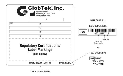
A=Medical/ICT/ITE/Household use Power Supply B=P/N: (料号) TR9KG2400CCPCIMR6B C=Model (型号) GTM96300-3619.5-4.5-T2 D=Input (输入)100-240V~, 50-60 Hz, 1A E=Output (输出)15.0 V == 2.4 A, 36.00W
