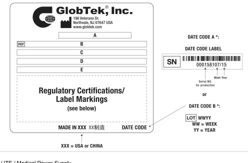
A=ICT / ITE / Medical Power Supply B=P/N: (料号) TR9KE9000LCP-IM(R6B) C=Model (型号) GTM961200P10812-T2 D=Input (输入)100-240V~, 50-60 Hz, 1.5 A E=Output (输出)12.0 V === 9.0 A, 108.00W
