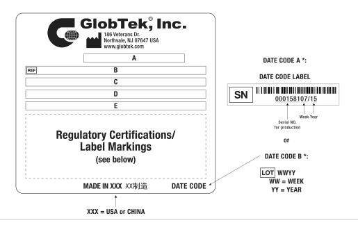
A=ICT / ITE / Medical Power Supply B=P/N: (料号) TR9KE9000CCP-IM(R6B) C=Model (型号) GTM961200P10812-T2 D=Input (输入)100-240V~, 50-60 Hz, 1.5 A E=Output (输出)12.0 V == 9.0 A, 108.00W
