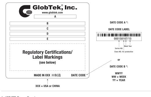
A=ICT/ITE Power Supply B=P/N: (料号) TR9KE5000LCP-N(R6B) C=Model (型号) GT-46600-6012-T2 D=Input (输入)100-240V~, 50-60 Hz, 1.5A E=Output (输出)12.0 V === 5.0 A, 60.00W
