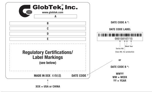
A=ICT/ITE Power Supply B=P/N: (料号) TR9KE5000CCP-N(R6B) C=Model (型号) GT-46600-6012-T2 D=Input (输入)100-240V~, 50-60 Hz, 1.5A E=Output (输出)12.0 V == 5.0 A, 60.00W
