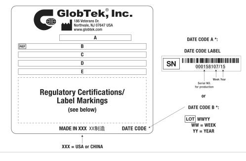
A=Medical/ICT/ITE/Household use Power Supply B=P/N: (料号) TR9KE3000T00-IMR6BG C=Model (型号) GTM96300-3614.5-2.5-T2 D=Input (输入)100-240V~, 50-60 Hz, 1A E=Output (输出)12.0 V === 3.0 A, 36.00W
