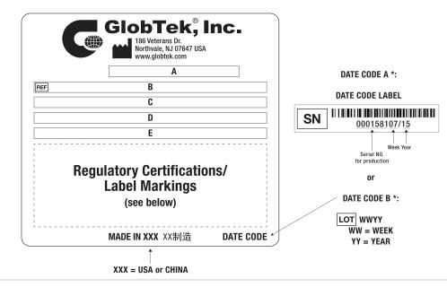
A=Medical/ICT/ITE/Household use Power Supply B=P/N: (料号) TR9KE3000LCPCIM(R6B) C=Model (型号) GTM96300-3614.5-2.5-T2 D=Input (输入)100-240V~, 50-60 Hz, 1A E=Output (输出)12.0 V === 3.0 A, 36.00W
