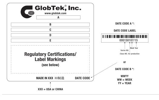
A=ICT/ITE Power Supply B=P/N: (料号) TR9KE2000LCP-N(R6B) C=Model (型号) GT-46240-2412-T2 D=Input (输入)100-240V~, 50-60 Hz, 0.6 A E=Output (输出)12.0 V === 2.0 A, 24.00W
