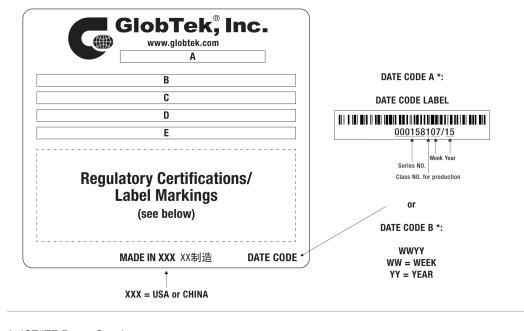
A=ICT/ITE Power Supply B=P/N: (料号) TR9KE1500LCP-N(R6B) C=Model (型号) GT-46181-1812-T2 D=Input (输入)100-240V~, 50-60 Hz, 0.5A E=Output (输出)12.0 V == 1.5 A, 18.00W
