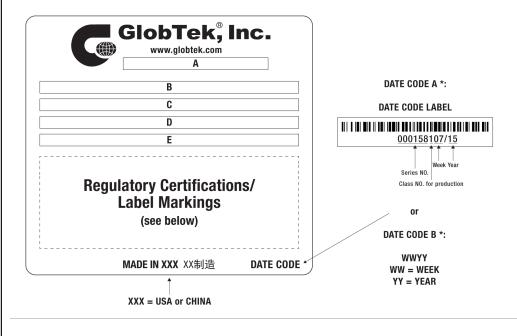
A=ICT/ITE Power Supply B=P/N: (料号) TR9KE1500CCP-N(R6B) C=Model (型号) GT-46181-1812-T2 D=Input (输入)100-240V~, 50-60 Hz, 0.5A E=Output (输出)12.0 V == 1.5 A, 18.00W
