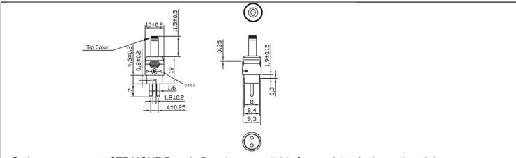
Option upon request: STRAIGHT Female Barrels are available for special order in any length between 9mm-14mm
