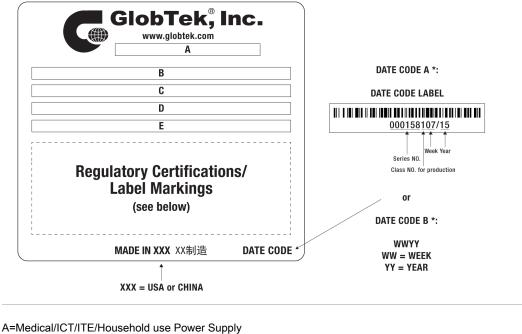
A=Medical/ICT/ITE/Household use Power Suppl B=P/N: (料号) TR9KD3333T00NAIMR6B C=Model (型号) GTM96300-3010.5-1.5-T2 D=Input (输入)100-240V~, 50-60 Hz, 1A E=Output (输出)9.0 V ---- 3.33 A, 30.00W
