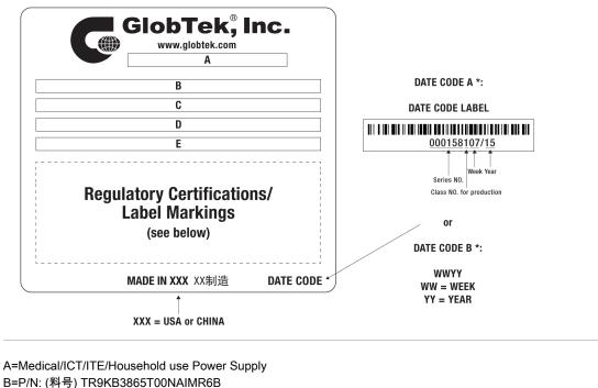
C=Model (型号) GTM96300-2307.5-1.55-T2 D=Input (输入)100-240V~, 50-60 Hz, 1A E=Output (输出)5.95 V --- 3.86 A, 23.00W
