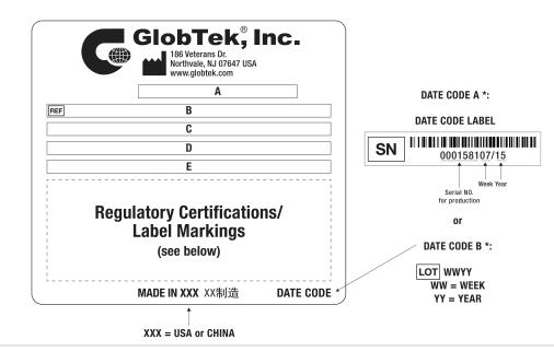
A=ICT / ITE / Medical Power Supply/Class 2/Household Power Supply B=P/N: (料号) TR9KA3600USBC-IMR6B C=Model (型号) GTM96180-1807-2.0-T2 D=Input (输入)100-240V~, 50-60 Hz, 0.6 A E=Output (输出)5.0 V ---- 3.6 A, 18.00W
