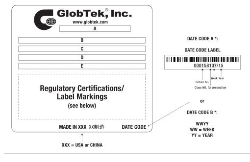
A=ICT/ITE Power Supply B=P/N: (料号) TR9KA3000CCP-N(R6B) C=Model (型号) GT-46181-1505-T2 D=Input (输入)100-240V~, 50-60 Hz, 0.5A E=Output (输出)5.0 V == 3.0 A, 15.00W
