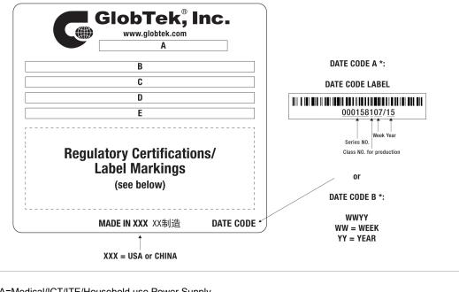
A=Medical/ICT/ITE/Household use Power Supply B=P/N: (料号) TR9CZ9470LRPIMR6B C=Model (型号) GTM961800P18019-T3 D=Input (输入)100-240V~, 50-60Hz, 2.2A E=Output (输出)19.0 V === 9.47 A, 180.00W
