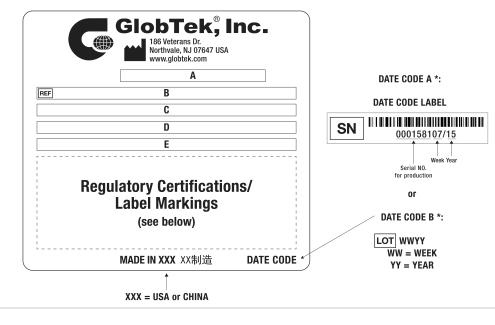
A=Medical/ICT/ITE/Household use Power Supply B=P/N: (料号) TR9CZ8421LCPIMR6B C=Model (型号) GTM961600P16019-T3 D=Input (输入)100-240V~, 50-60 Hz, 2.2A E=Output (输出)19.0 V === 8.42 A, 160.00W
