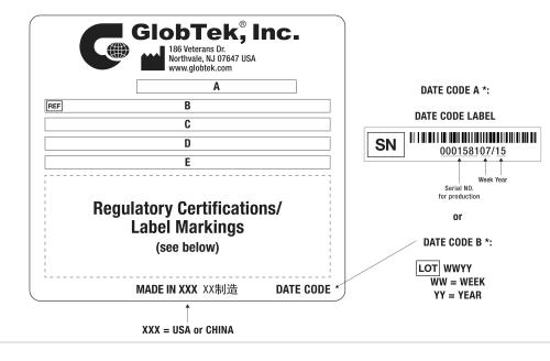
A=USB Adaptive Power Source ICT/ITE/Medical Power supply B=P/N: (料号) TR9CZ5000USBCJG2R6BF2 C=Model (型号) GTM961005P-100PD-USBCJ–T3 D=Input (输入)100-240V~, 50-60Hz, 1.5A
