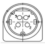
PIN 1,2: +V Pin 1,2: +V, Shell, Pin 3, 4: Common/Ground
