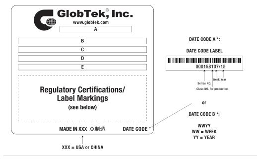
A=ICT/ITE Power Supply B=P/N: (料号) TR9CZ2105CCP-N(R6B) C=Model (型号) GT-46400-4019-T3 D=Input (输入)100-240V~, 50-60 Hz, 1.0A E=Output (输出)19.0 V == 2.1 A, 40.00W
