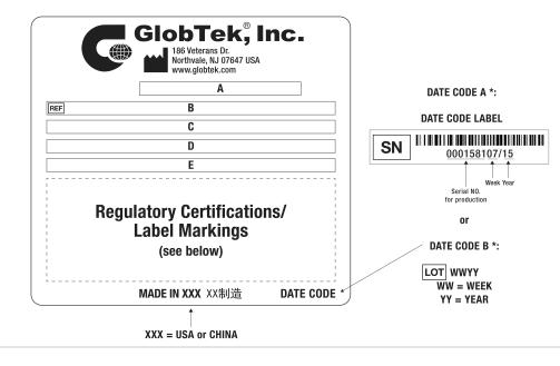
A=USB Adaptive Power Source ICT/ITE/Medical Power supply B=P/N: (料号) TR9CZ1800USBCFG2R6B C=Model (型号) GTM96181-36PD-T3 D=Input (输入)100-240V~, 50-60 Hz, 1.2A
