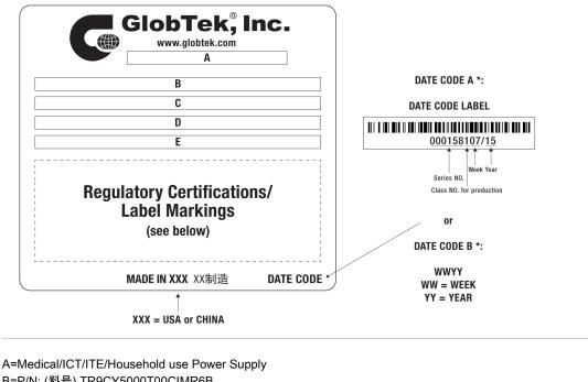
B=P/N: (料号) TR9CY5000T00CIMR6B C=Model (型号) GTM961800P18036-T3 D=Input (输入)100-240V~, 50-60Hz, 2.2A E=Output (输出)36.0 V === 5.0 A, 180.00W
