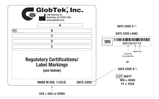
A=Medical/ICT/ITE/Household use Power Supply B=P/N: (料号) TR9CX3333T00-IMCF(R6B) C=Model (型号) GTM961800P18054-T3-CF D=Input (输入)100-240V~, 50-60Hz, 2.2A E=Output (输出)54.0 V == 3.33 A, 180.00W
