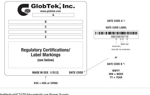
A=Medical/ICT/ITE/Household use Power Supply B=P/N: (料号) TR9CX3333LRPIMR6B C=Model (型号) GTM961800P18054-T3 D=Input (输入)100-240V~, 50-60Hz, 2.2A E=Output (输出)54.0 V === 3.33 A, 180.00W
