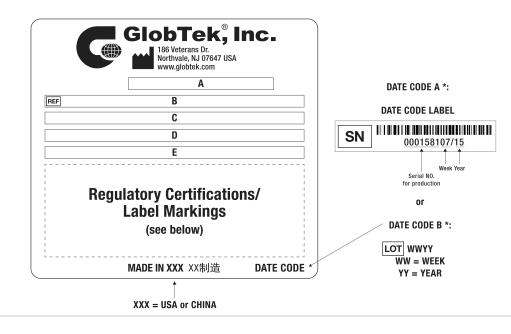
A=ICT / ITE / Medical Power Supply/Class 2/Household Power Supply B=P/N: (料号) TR9CR3000T00-IM(R6B) C=Model (型号) GTM96900P9030-T3 D=Input (输入)100-240V~, 50-60Hz, 1.5A E=Output (输出)30.0 V === 3.0 A, 90.00W
