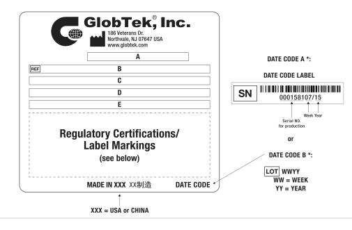
A=ICT / ITE / Medical Power Supply/Class 2/Household Power Supply B=P/N: (料号) TR9CR2160T00IMCFR6B C=Model (型号) GTM96600-6530-T3-CF D=Input (输入)100-240V~, 50-60Hz, 1.5A E=Output (输出)30.0 V === 2.16 A, 65.00W
