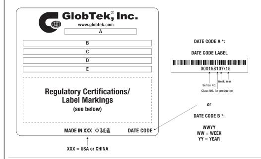
A=ICT / ITE / Medical Power Supply B=P/N: (料号) TR9CN8200LRP-IM(R6B) C=Model (型号) GTM961200P11113.5-T3 D=Input (输入)100-240V~, 50-60 Hz, 1.5 A E=Output (输出)13.5 V == 8.22 A, 111.00W
