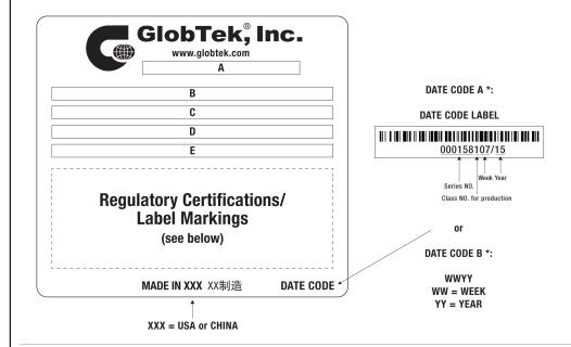
A=ICT / ITE / Medical Power Supply/Class 2/Household Power Supply B=P/N: (料号) TR9CI750CRLPCIM(R6B) C=Model (型号) GTM96180-1830-6.0-T3 D=Input (输入)100-240V~, 50-60 Hz, 0.6 A E=Output (输出)24.0 V == 0.75 A, 18.00W
