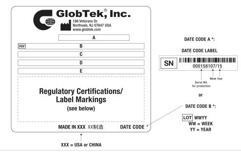
A=Medical/ICT/ITE/Household use Power Supply B=P/N: (料号) TR9CI7500A00CIMCFR6B C=Model (型号) GTM961800P18024-T3-CF D=Input (输入)100-240V~, 50-60Hz, 2.2A E=Output (输出)24.0 V == 7.5 A, 180.00W
