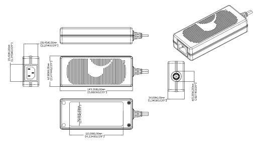
Alternative housing with input cord clamp to prevent accidental removal of the power cord. Product PN# ends with suffix "CL"
