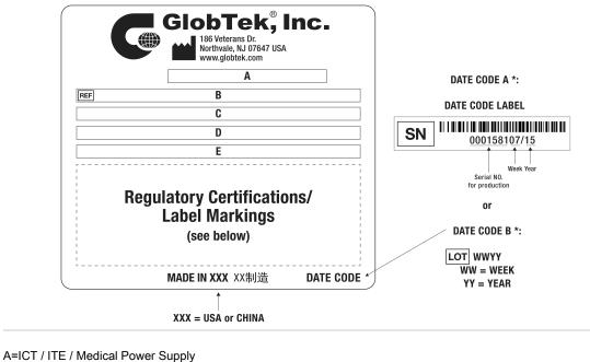
A=ICT / ITE / Medical Power Supply B=P/N: (料号) TR9CI5000T00-IM(R6B) C=Model (型号) GTM961200P12024-T3 D=Input (输入)100-240V~, 50-60 Hz, 1.5 A E=Output (输出)24.0 V === 5.0 A, 120.00W
