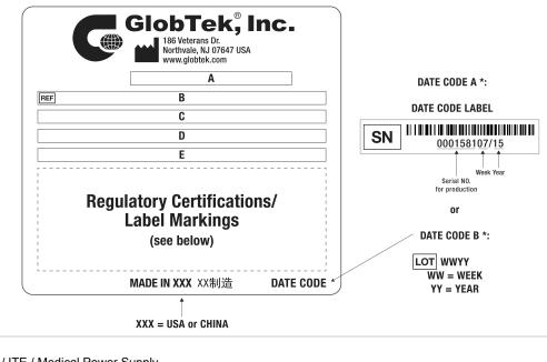
A=ICT / ITE / Medical Power Supply B=P/N: (料号) TR9CI5000CCP-IM(R6B) C=Model (型号) GTM961200P12024-T3 D=Input (输入)100-240V~, 50-60 Hz, 1.5 A E=Output (输出)24.0 V === 5.0 A, 120.00W
