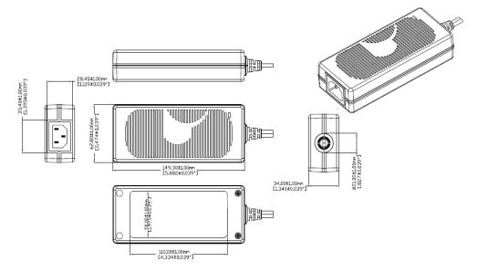
Alternative housing with input cord clamp to prevent accidental removal of the power cord. Product PN# ends with suffix "CL"
