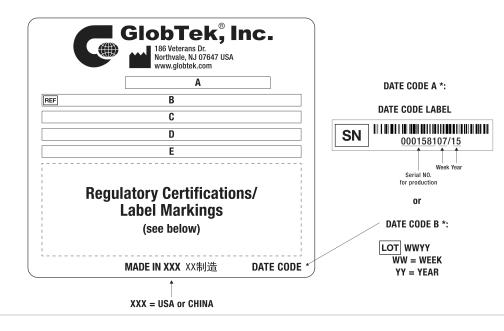
A=ICT / ITE / Medical Power Supply/Class 2/Household Power Supply B=P/N: (料号) TR9CI3750LCPIMR6BLPS C=Model (型号) GTM96900P9024-T3Z D=Input (输入)100-240V~, 50-60Hz, 1.5A E=Output (输出)24.0 V === 3.75 A, 90.00W
